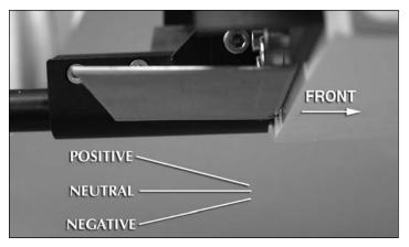
You can use a large pair of pliers to adjust the trim plates. Remember, just tweak the plates as a very small adjustment can drastically change the way the boat runs.
