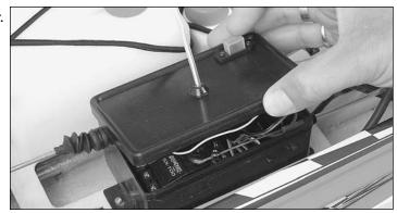
$\square$  9. Using the screwdriver, carefully pry the retainer over the tabs.
