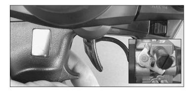
□ 5. Off or stop position. If this is not the case, move the steering servo reverse switch located on the front of the transmitter (2) to the other position. Note: You might have to readjust the position of the throttle arm of the throttle servo to properly get the carburetor to match the pictures.
