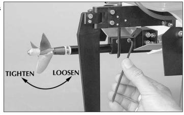
Slide the inner strut assembly with shaft out of the boat. Wipe away any oil and grease.
