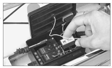
☐ 8. Replace the radio box cover and radio box lid retainer. Use your screwdriver to install the retainer.
