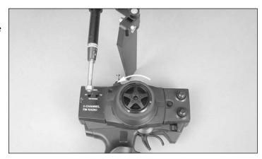
☐ 2. Move the steering wheel to the right. The back rudder should move to the right. If this is not the case, simply move the steering servo reverse switch located on the front of the transmitter (2) to the other position.
