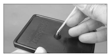
☐ 5. It is only necessary to push the antenna in to the point it is even with the back side of the cover.
