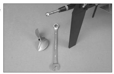
☐ 2. Install the propeller on the shaft; replace the nut, making sure it is tight.
