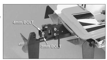
$\square$  2. Insert the rudder into the rudder control arm assembly as shown. Replace the 4 x 15mm screw and 3 x 15mm screw and secure them with the 4mm and 3mm nuts, respectively.
