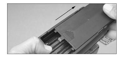
☐ 2. Install eight (8) fresh "AA" batteries into the bottom of the transmitter in the configuration molded into the battery holder.
