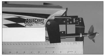
**Negative Propeller Thrust:** Causes the bow to run low (flat on the water). This reduces speed and may cause the boat to stuff (crash by having the boat's bow tuck under water).
