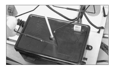
☐ 4. Slide the receiver antenna into the top of the radio box cover by gently pushing it in place.
