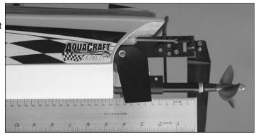
**Positive Propeller Thrust:** This setting causes the bow to run high. This makes the boat run faster but looser at the same time. In rough water this can cause the boat to blow off (crash by having the bow of the boat lift off the water).
