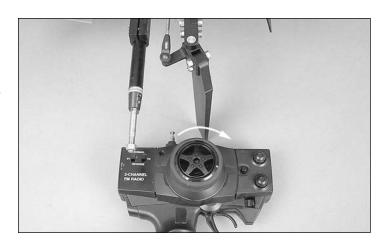
☐ 3. Squeeze the throttle trigger on the transmitter; this should open the throat of the carburetor. This is the proper throttle arm position for full throttle.
