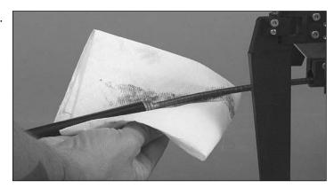
Re-grease the shaft using GrimRacer Speed Grease. Re-install the shaft and inner strut housing, making sure the two 4mm screws are tight.
