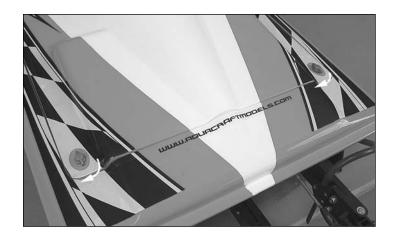
☐ 2. Using a standard screwdriver, remove the wire radio box lid retainer by gently prying the wire over the holding tabs on the side of the box.
