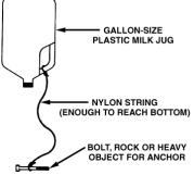
• Make 2 to 4 simple and inexpensive "marker buoys" with empty milk jugs, string, and heavy objects for anchors, similar to the above sketch.
