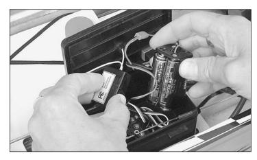
☐ 7. Replace the battery holder inside the radio box. Make sure that it will not interfere with any of the control linkages.
