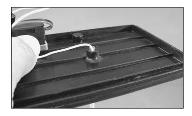
☐ 6. Place four (4) new "AA" batteries into the receiver battery holder. Be sure to follow the polarity diagram molded into the battery holder.
