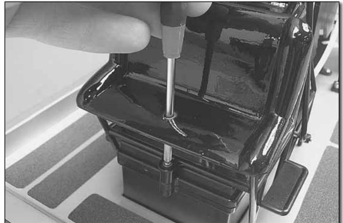
❑ 1. Using a #1 Phillips screwdriver (small), remove the two (2) Phillips head screws from the top of the radio box. One is located under the front seat of the boat and the other behind the back seat.
