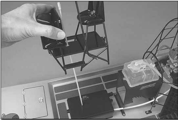
❑ 2. Remove the seat assembly as well as the top of the radio box and lay them to the side.
