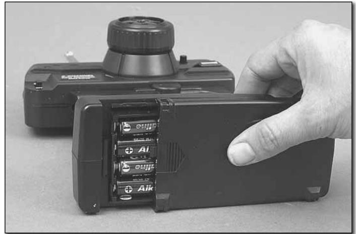
❑ 4. Reinstall the battery door onto the bottom of the transmitter.
