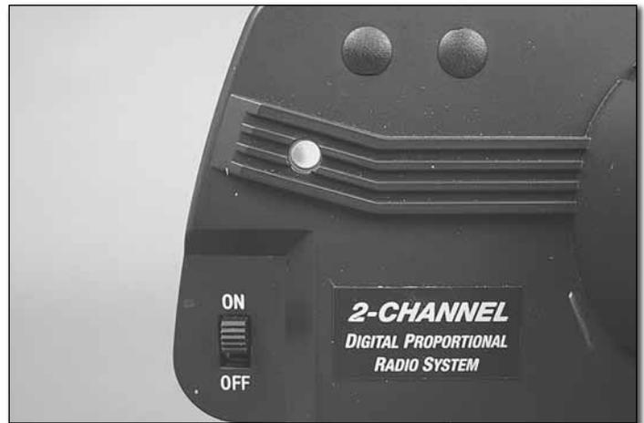
❑ 5. Turn the transmitter "ON" using the switch on the transmitter's left side. The battery level indicator light (LED) should glow green. If the light is flashing the batteries are low and need to be replaced.
