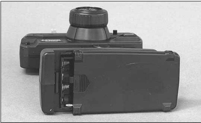
❑ 2. Slide off the battery door from the bottom of the transmitter.
