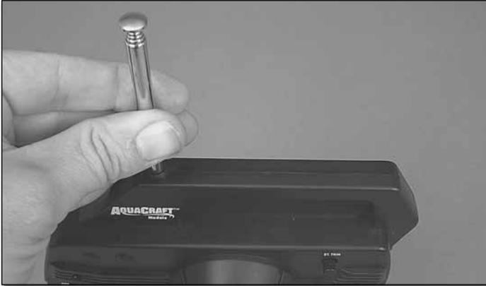
❑ 1. After removing the transmitter and transmitter antenna from the box, line up the antenna to the hole in the top of the transmitter. Slip the antenna in and lightly screw the antenna into the transmitter. Do not over tighten. Give the antenna a light tug to make sure it is properly installed.
