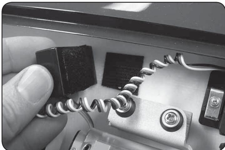
**1.** Mount your receiver in your boat by installing hook and loop to the bottom of your receiver. Install the receiver in the position shown in the picture.
