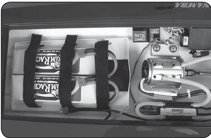
**2.** Remove the canopy and install the batteries, making sure they are well strapped in and seated.
