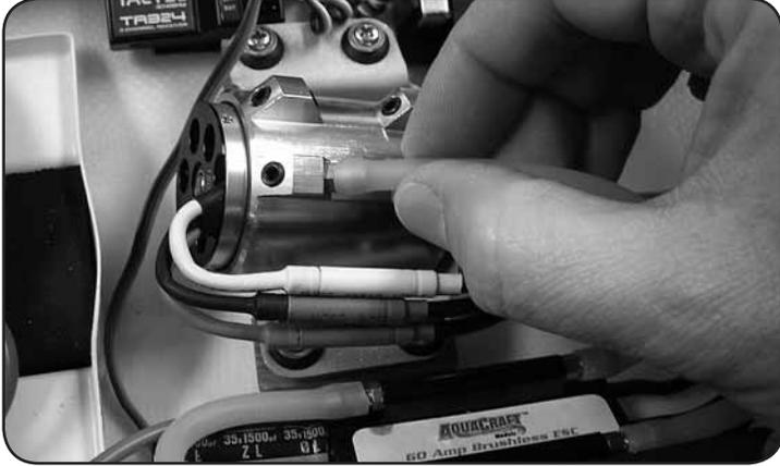
**1.** Start by removing the water lines to the motor jacket. Also unplug the three connector leads to the motor.
