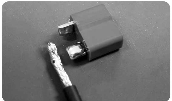
**1.** Begin by tinning (pre-applying) solder to both the positive and negative solder tabs on the Deans connector; also remove about 3/4" of insulation off one end of the length of wire and tin the exposed wire as well.
