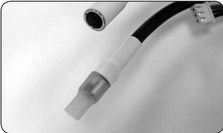
**10.** Cut a 3/4" long length of fuel tubing and slide it over the end of the connector of the back battery connector. **NOW, WHEN THE BATTERY IS NOT IN USE, ALWAYS STORE AND KEEP THIS TUBING OVER THE CONNECTOR. DO NOT REMOVE THE TUBING FOR ANY REASON EXCEPT CHARGING AND OPERATING.**
