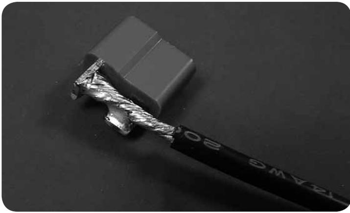
**2.** Solder the wire across the two solder tabs, creating a bridge between the two tabs. Use your side cutters to remove the excess wire.
