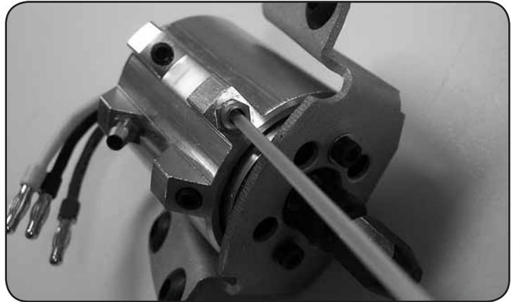
**5.** Place the motor in a rag or paper towel and spray a water displacer into the fittings on the water jacket as well as in the motor itself. After the motor is "pickled," wipe it down and reinstall it in the boat using the above instructions in reverse order.
