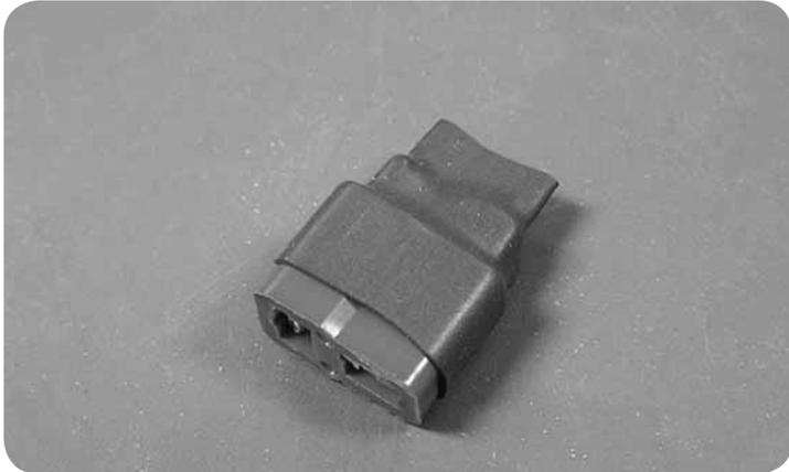
**3.** Cut the shrink tube to around 1" long and place over the connector and exposed solder work. Shrink the tubing and with the tube still warm pinch the end closed.
