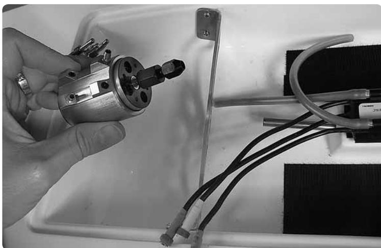
Remove the motor from the boat.
