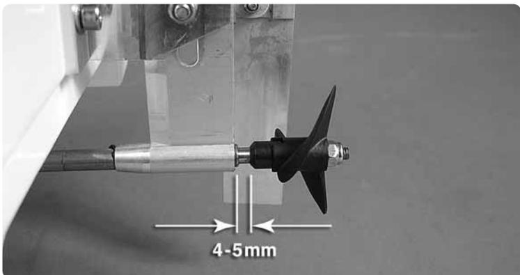
Before tightening the cable coupler, make sure to leave 4 or 5mm distance between the back of the strut and the front of the drive dog. This will keep the drive system from binding or breaking as the cable retracts during operation. Tighten the cable coupler, reversing the direction of the open end wrenches. **DO NOT OVER TIGHTEN.**
