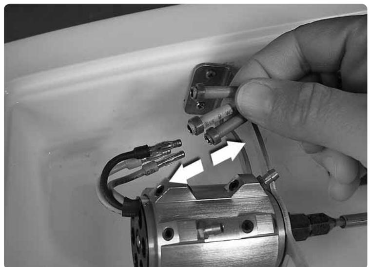
Unplug the three 4mm connector leads to the motor.
