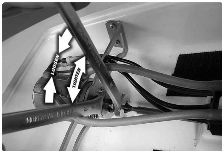
Loosen the cable coupler using the 10mm and 12mm wrenches.
