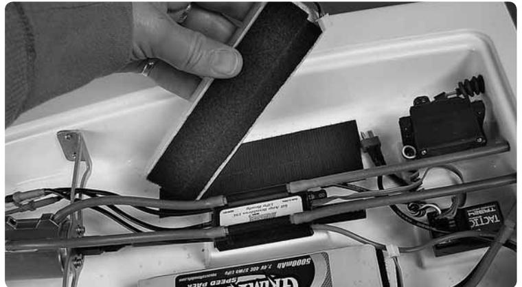
Remove the canopy and install the provided hook and loop material to your battery packs. Install the batteries, making sure they are well seated.
