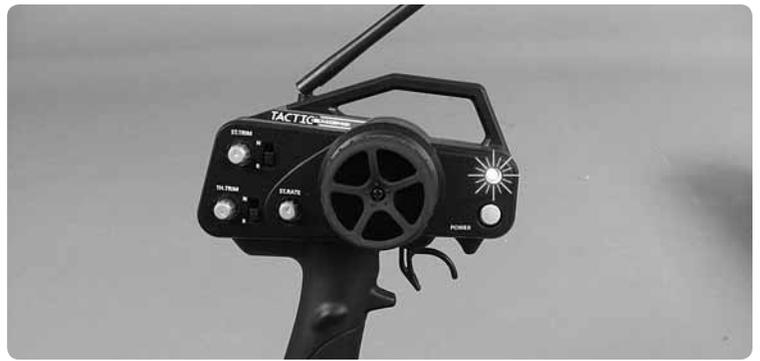
Turn on the transmitter, making sure it's working by viewing the LED on the front. The LED should glow bright red.
