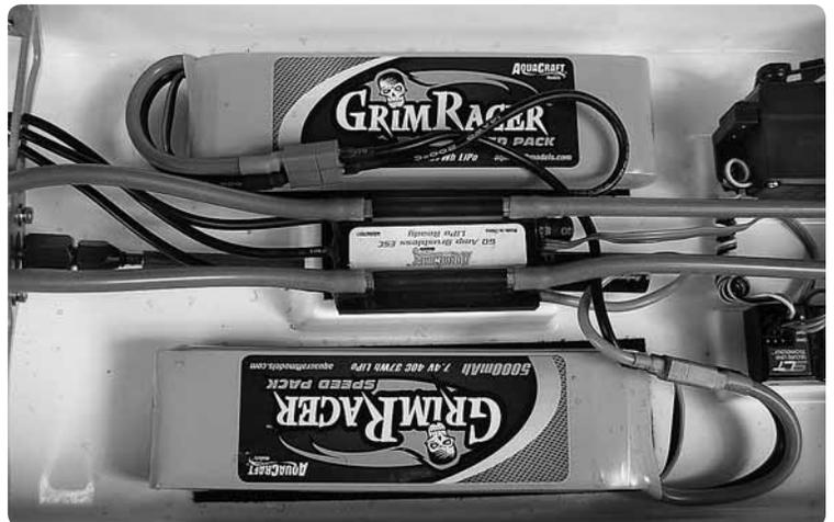
Stand clear of the propeller and plug each of the battery packs into the motor controller.
