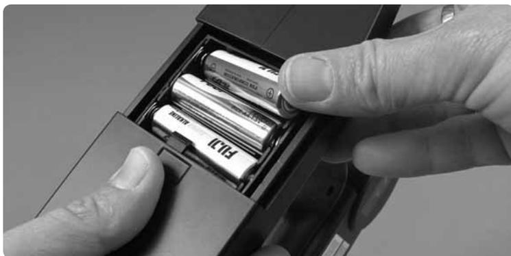
Install 4 AA batteries into the transmitter using the installation pattern molded into the bottom of the battery tray.
