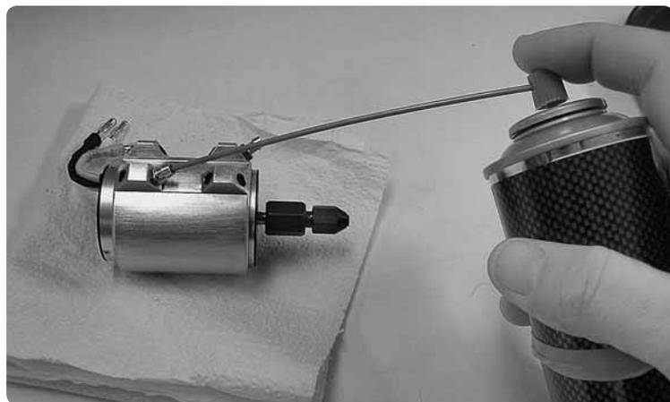
After the motor is "pickled," wipe it down and reinstall it in the boat using the above instructions in reverse order.
