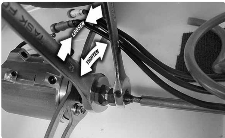
Use the 12mm and 10mm wrenches to loosen the cable coupler from the cable. To do so, hold the 12mm wrench still and rotate the 10mm wrench counterclockwise.
