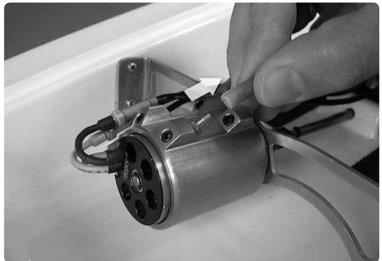
Start by removing the water lines to the motor jacket.
