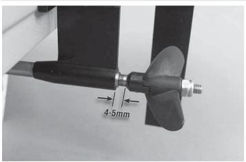
Before tightening the cable coupler, make sure to leave a 4 or 5mm distance between the back of the strut and the front of the drive dog. This will keep the drive system from binding or breaking as the cable operates. Tighten the cable coupler, reversing the direction of the open end wrenches. **DO NOT OVERTIGHTEN.**
