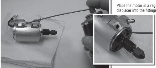
Place the motor in a rag or paper towel and spray a water displacer into the fittings on the water jacket as well as in
