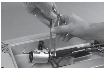
Fully loosen the coupler. Using a rag cover the prop and firmly pull the prop and shaft away from the coupler. Use a 2.5mm hex wrench to loosen the two motor screws.
