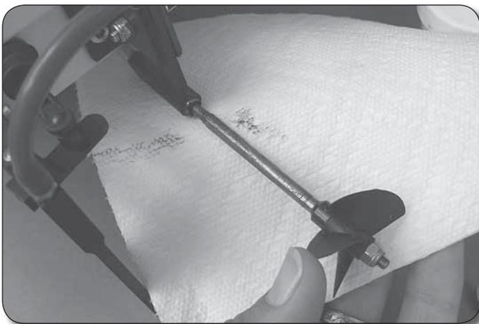
3. Slide the shaft out from the back of the boat and re-grease. Reinstall and retighten the cable.
