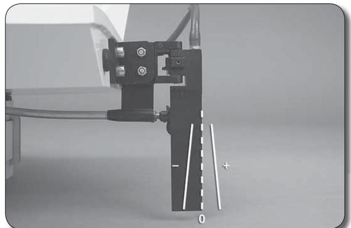
**RUDDER** – You can tilt the rudder fore and aft to change the way the boat handles. The more you tuck the rudder under the boat (negative angle), the tighter the boat runs on the water. Tilting it back (positive angle) causes the back of the boat to run looser. You don't want to overdo it so just work within the amount of movement provided by the bolts. Also the more you tilt the rudder back the less aggressive the steering becomes.
