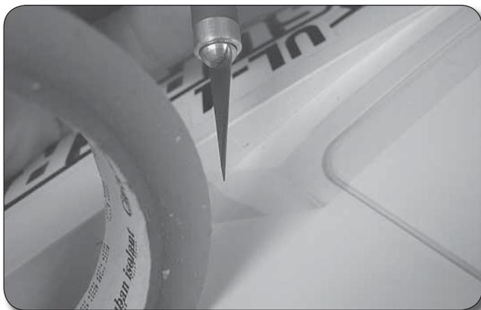
5. Tape the cowl in place carefully, making sure you press it securely down. Make sure you use a good quality hatch tape like GrimRacer Pro Radio Box Tape. Other radio box tapes can leave sticky adhesive that can be hard to remove.
