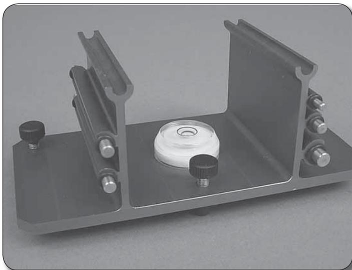
To maximize performance — and minimize damage to on-board electronics and parts — balance your props with the GrimRacer Precision Prop Balancer. It's easy to use. Three thumb screws provide perfect level adjustment, and a precise bubble level is built into the one-piece extruded aluminum base. The balancer includes balancing shafts for 1/8" (3.2 mm), 3/16" (4.8 mm) and 1/4" (6.4 mm) bore prop hubs. Propeller not included. **AQUB9575**
