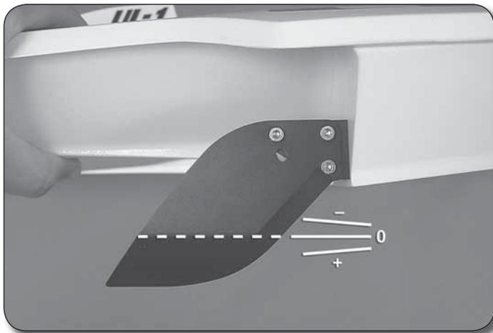
**TURN FIN** – The turn fin is what holds the boat in the corners at speed. The turn fin can also be tilted back and forth to change the way the boat handles. Tilting the fin up (positive) causes the boat to run tighter on the water and tilting it down (negative) causes it to run looser.
