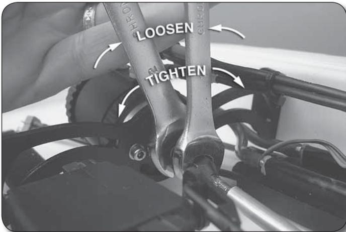
2. To loosen the cable coupler hold the 12mm wrench still and turn the 10mm wrench counterclockwise. To tighten turn the 10mm wrench clockwise.
