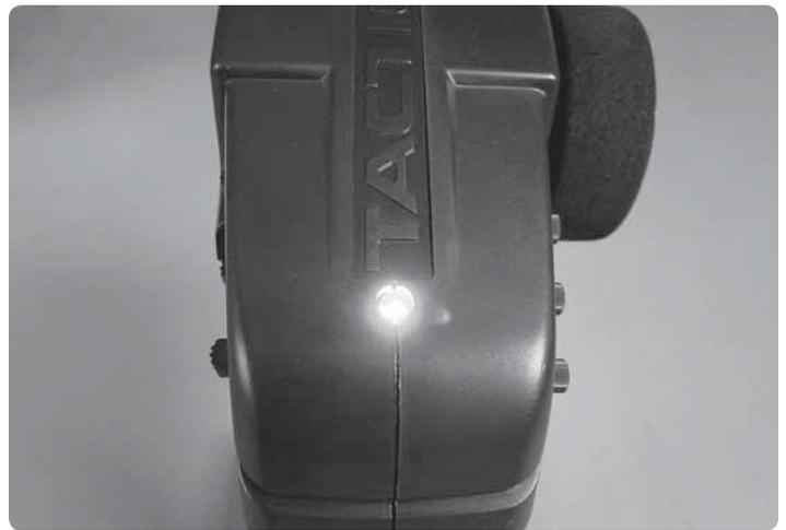
Turn the transmitter on by pressing the "Power" button on the right side of the transmitter. The battery indicator light (LED) should glow green. If the light is flashing, the batteries are low and need to be replaced.
