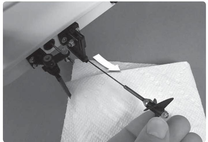
Slip the driveshaft out the back of the boat. Wipe off any grease and water that might be on the shaft. Using GrimRacer Speed Grease, apply a small amount to the shaft and slide it back into the boat. Be careful to align the driveshaft to the hole in the end of the motor coupler.
