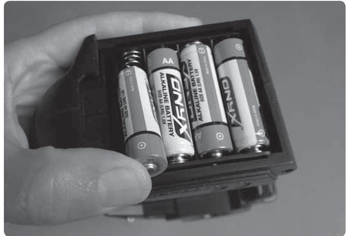
Install 4 "AA" batteries into the transmitter in the configuration molded into the battery floor and reinstall the battery door.
