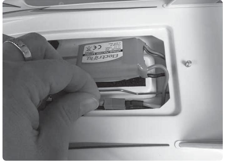
Tuck the wires neatly under the decking.
