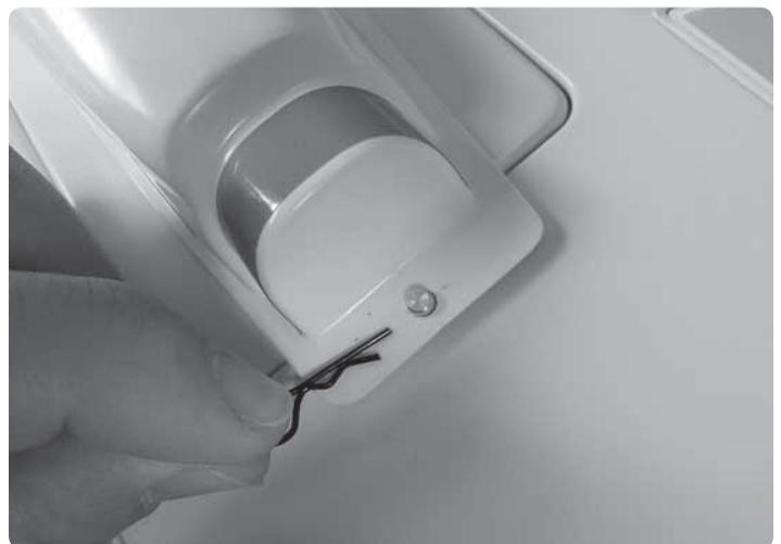
Turn on your transmitter. Remove the main canopy by pulling the pin on the back of the cowl.
