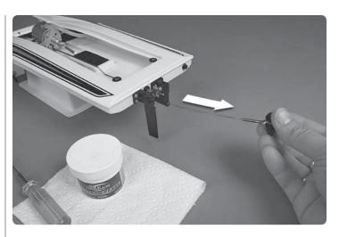
Slip the driveshaft out the back of the boat. Wipe off any grease and water that might be on the shaft.
