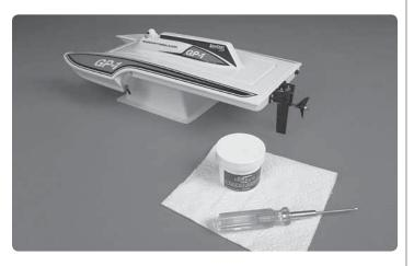
It is important to remove and re-lubricate the driveshaft after running for the day. Make sure the battery pack is unplugged. You will need a 2mm hex wrench, GrimRacer Cable Grease and some paper towels.
