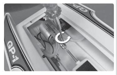
Using a 2mm hex wrench, loosen the screws holding the drive cable to the motor coupler. It is important to note that there are two set screws holding the shaft in position.
