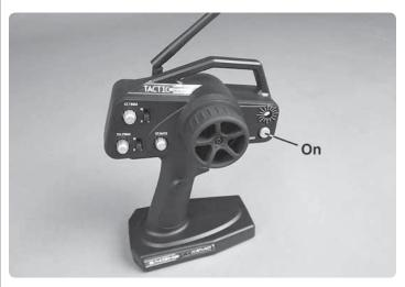
Turn the transmitter on by pressing the "Power" button on the right side of the transmitter. The battery indicator light (LED) should glow red. If the light is flashing, the batteries are low and need to be replaced.
