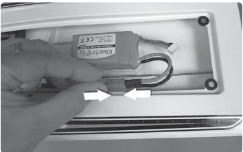
In your boat, you will find a length of hook and loop material on the battery tray. Remove the piece of hook and loop and install on to the battery's back. Install the battery into the boat as shown.
