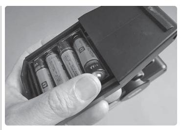
Install 4"AA" batteries into the transmitter in the configuration molded into the battery floor and reinstall the battery door.
