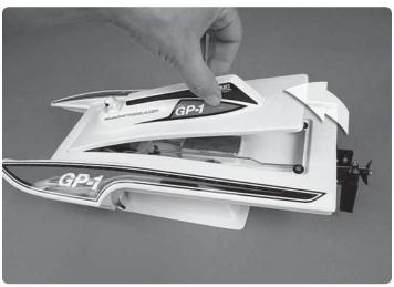
Remove the canopy by lifting at the back and rotating up off the front pins.
