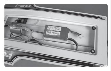
Tuck the wires neatly under the decking.
