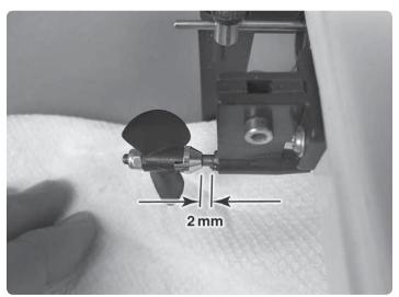
Leave about a 1/16" [2mm] gap between the front of the drive dog and the back of the brass tube. Retighten the shaft coupler screws.
