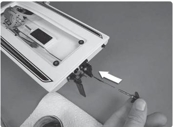
Using GrimRacer Speed Grease, apply a small amount to the shaft and slide it back into the boat. Be careful to align the driveshaft to the hole in the end of the motor coupler.
