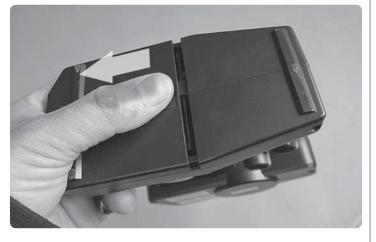
Slide off the battery door from the bottom of the transmitter.
