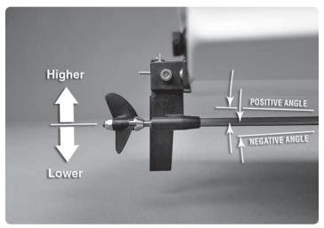
The strut can be *tweaked* to change the ride of the boat but only experienced modelers should attempt this. If you are going to *tweak* the strut remove the prop shaft and prop. Loosen the strut bolt. Move or adjust the strut, taking care not to lose the
