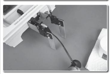
Using GrimRacer speed grease, apply a small amount to the shaft and slide the cable back into the boat. Be careful to align the drive shaft to the hole in the end of the motor coupler.
