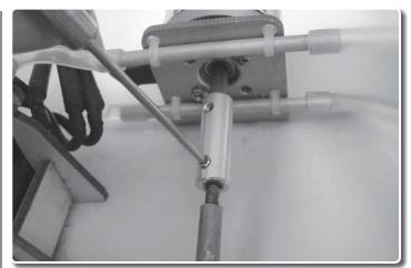
Now is also a good time to place a drop of light oil on the motor bearing.
