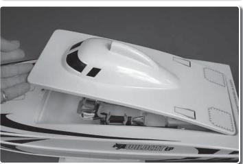
Install the battery pack by strapping it in place using the provided hook and loop material.
