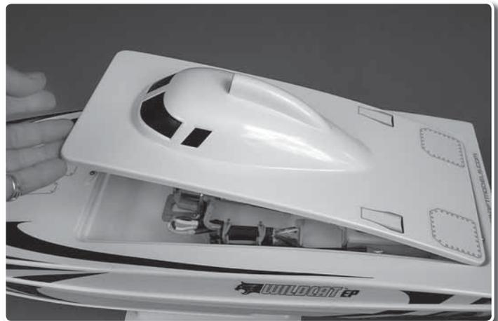
Install the battery pack by strapping it in place using the provided hook and loop material.
