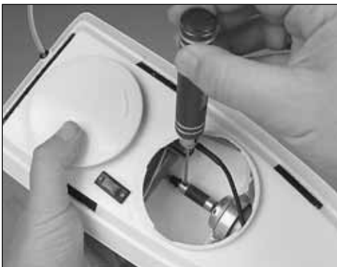
Loosen the aft 1.5mm set screw located on the motor/driveshaft coupler.
