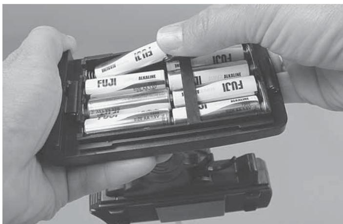
Install eight "AA" batteries into the bottom of the transmitter.
