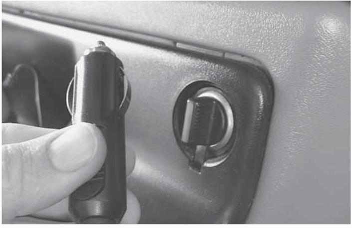
Plug the charger into a car power socket. The charger will start beeping and the light will flash. Connect the battery pack to the battery end of the charger. The charger will stop beeping and the light will stop flashing. You will know charging is complete when the charger starts to beep again and the light begins to flash.
