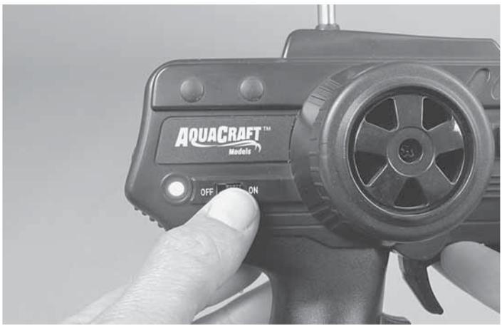
Install the transmitter antenna into the top of the transmitter, turning it clockwise to screw it in place. Then, turn the transmitter on, making sure the power light is glowing.
