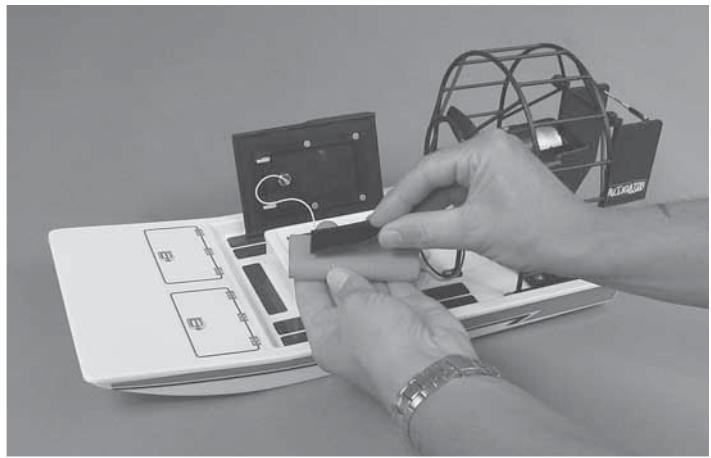
Place the charged battery into the open compartment and plug the battery into the boat.
