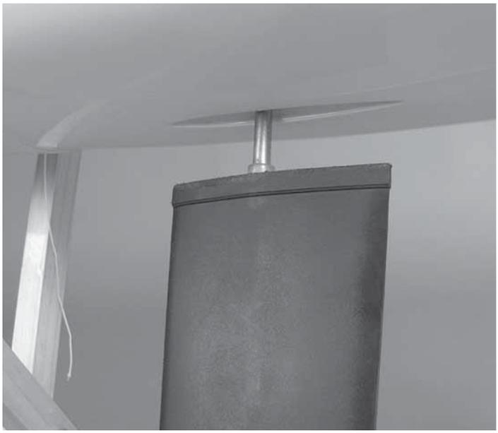
Slip the keel into the hole in the bottom of the hull.
