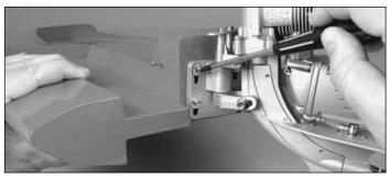
■ 8. Attach the engine to the transom with 6-32 socket head cap screws and #6 washers. **Do not tighten them completely at this time.**
